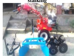
Attachments of mini power tiller cultivator, ridger and rotavator from left to right
